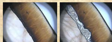
Figure 2a & b Dextran at -11.4°C and -9.1°C respectively
